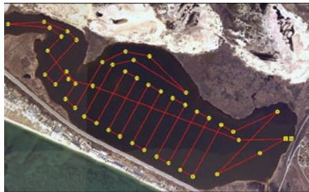
Screenshot from VectorMap mission planning software showing a "lawnmower"-style mission path drawn onto image of saltwater lagoon.
